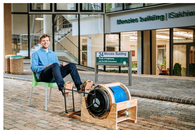
Kai Goodall and his Pedal 'n Spin foot cranked washing machine
