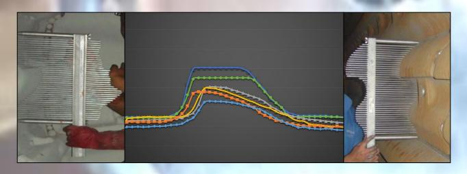
MPTech currently has new stock of their mechanical liner profile gauges. The gauges use aluminium pins to trace a profile of your installed or new liner/lifters. Once the profile is obtained the measurements can easily be transferred to a spreadsheet template (supplied) for further calculations.
