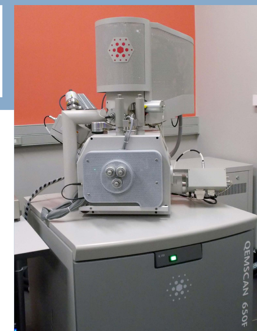
QEMSCAN 650F (right) and sample block holder with 30mm sample disks (left)
