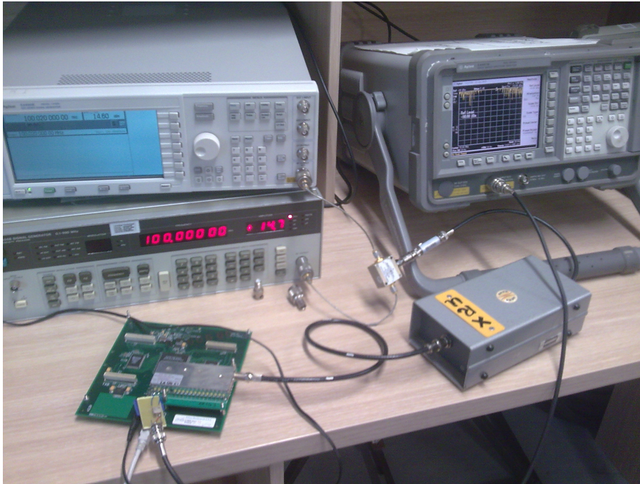
Figure 3.10: A picture of the experimental setup that was used to determine the IP_3 of the receiver.
