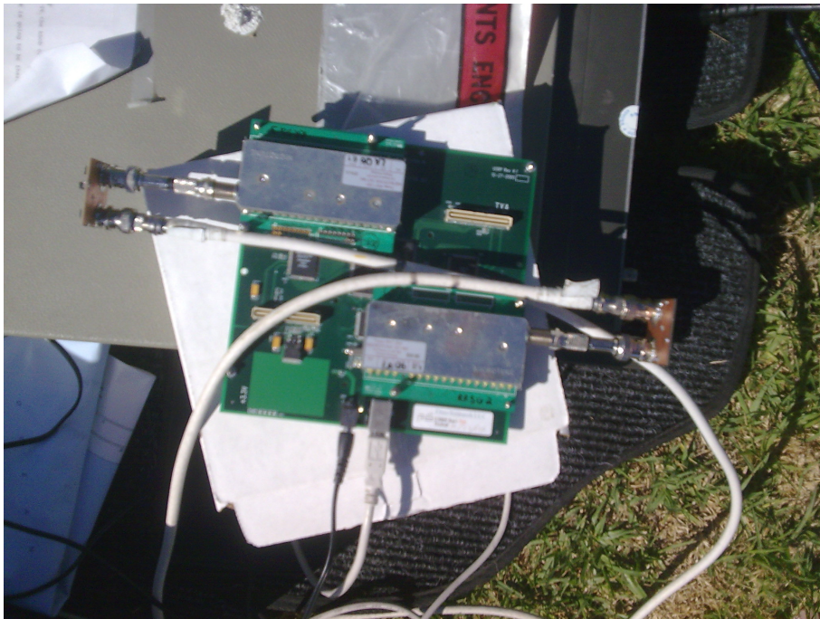
Figure 7.4: The USRP setup, showing two TVRX daughterboards and two bandpass filters, as well as the cables coming from the antennas.
