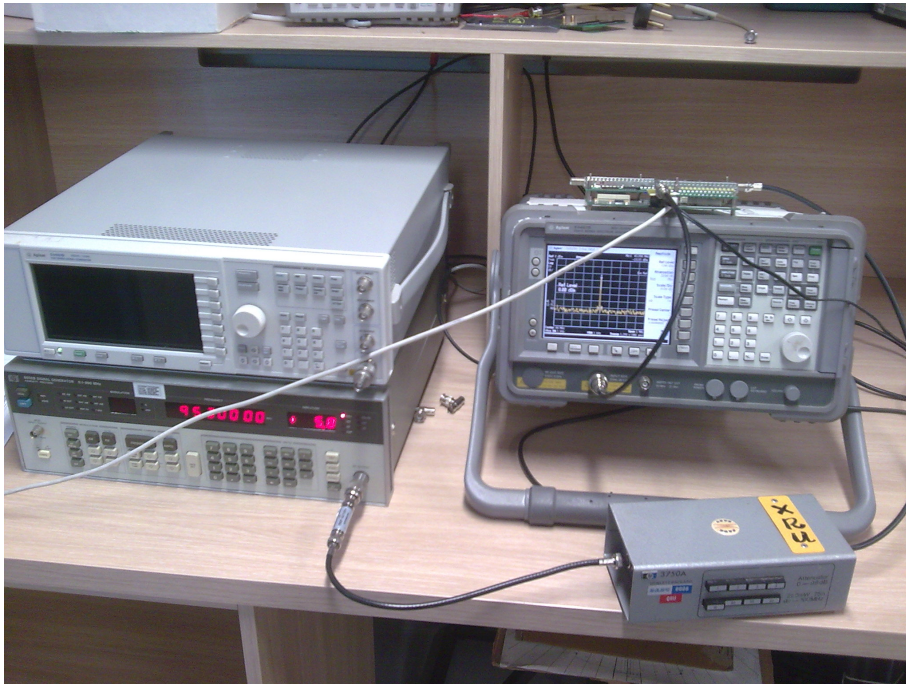
Figure 3.4: A picture of the experimental setup that was used to determine the 1-dB compression point of the receiver.
