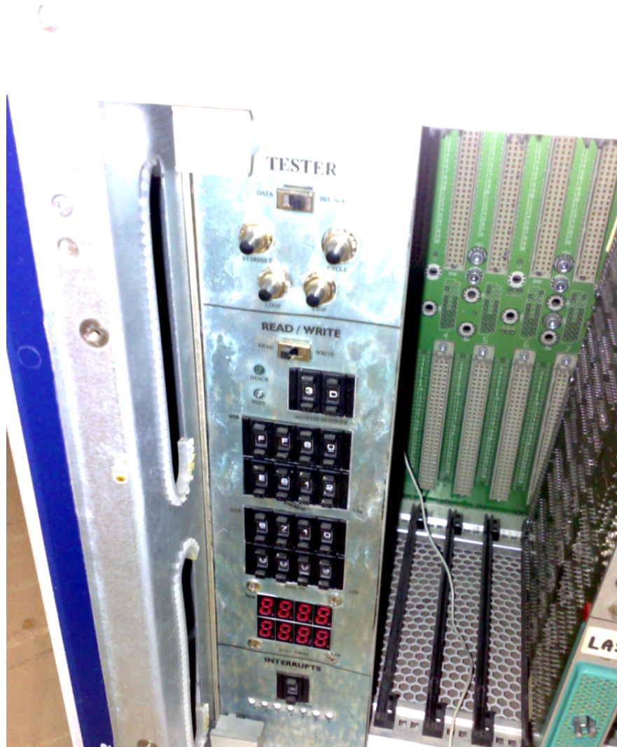
Figure 1.2: Front panel of the previous VMEbus tester, with all control switches. The switches were used to carry out VMEbus operations.
