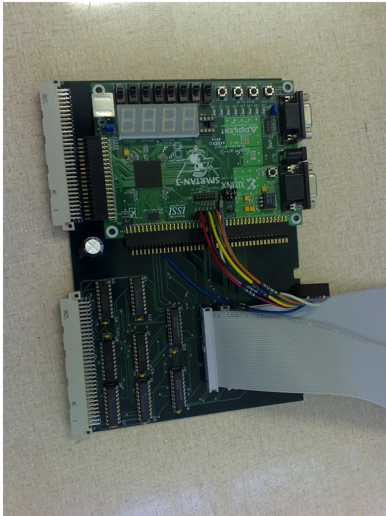
Figure 4.5: A complete implementation of exerciser hardware. Interface logic module and Spartan 3 development board are integrated into a single unit of 6U double-slot system.
