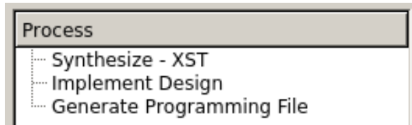
Figure 4.11: Compilation Menu: a screenshot illustrating the compilation options offered in the ROME environment.
