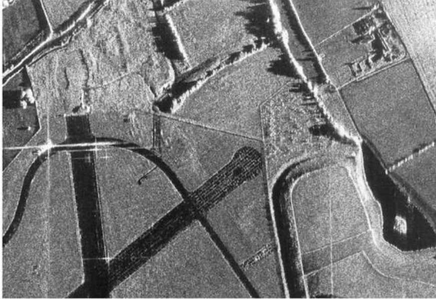
Figure 2.3: Example of a SAR image of farmland, generated with a resolution of one foot. Taken from Stimson [7].
