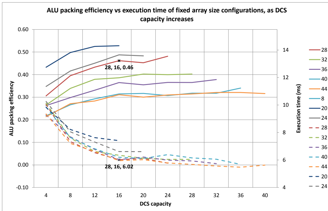
Figure 5.18 – In solid lines ALU packing efficiency for a limited range of array sizes is shown. On the second vertical axis and in dashed lines the corresponding execution times for the test case seven body system are shown. The horizontal axis represents the progressive increase in DCS capacity. Labels in the graph indicate in order, array size in Strips (series), DCS capacity (category), axis appropriate value
