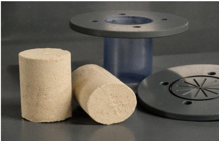
Figure 1: bio-columns grown from synthetic urine (Henze, 2017).
