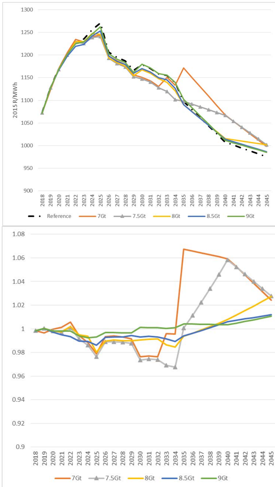
Figure 5: Effect on the electricity price of various GHG emissions budgets 2015 ZAR/MWh above and indexed to reference scenario below
