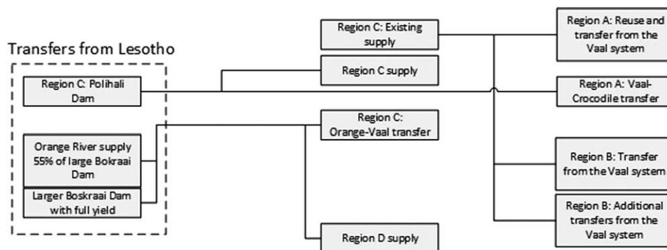
Figure 7. Schematic of the regional water supply network incorporated in SATIM-W.
