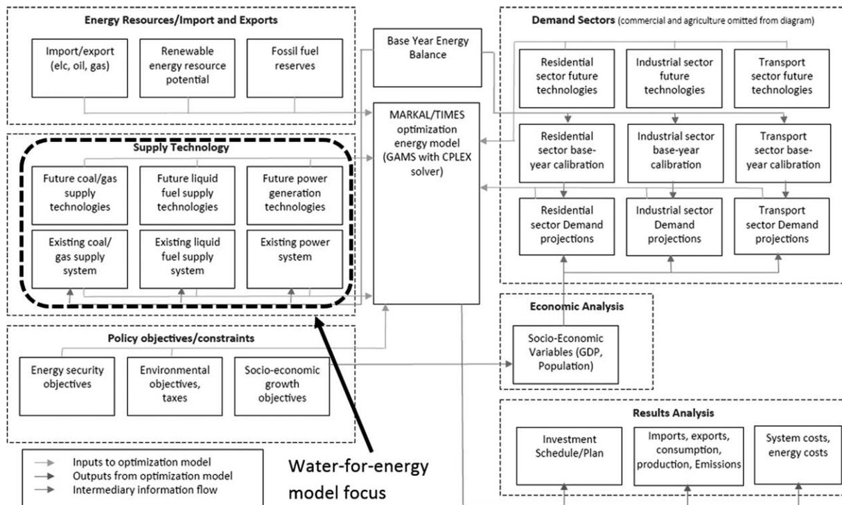
Figure 4. A process flow schematic of the SATIM energy systems model with the water-for-energy development focus highlighted.
