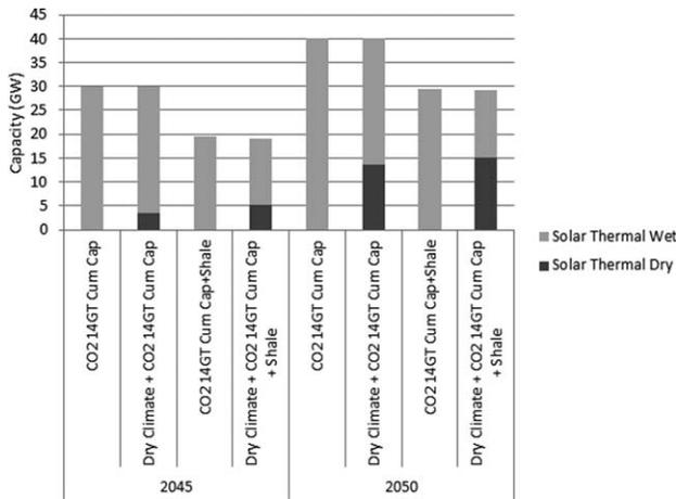
**Figure 22.** Installed capacity of solar thermal power plants (CSP) by cooling method.
