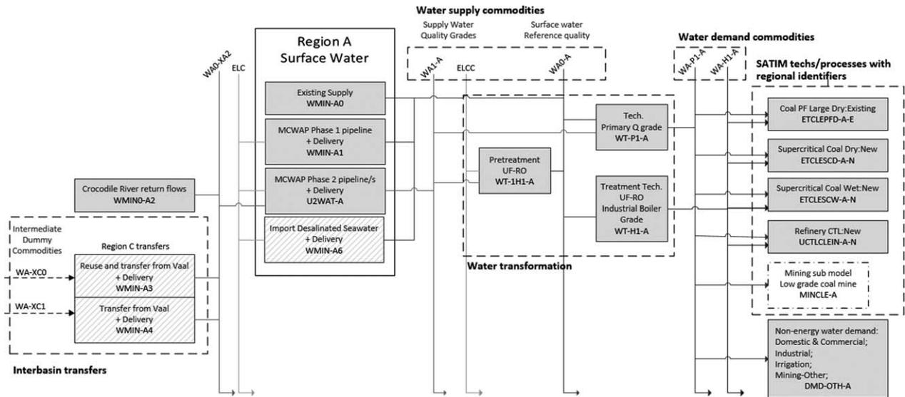
Figure 9. Incorporating water supply infrastructure in SATIM-W.
