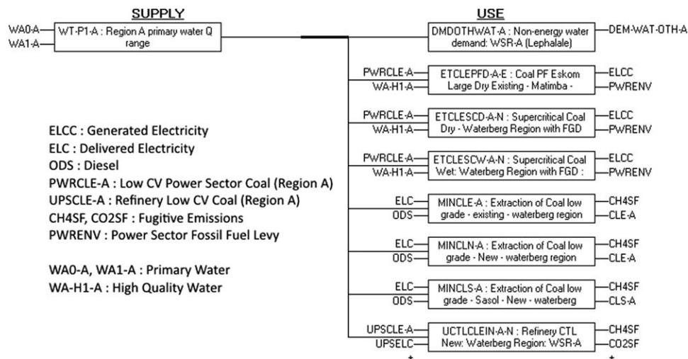
Figure 10. Water supply to regional technologies and processes in water supply region A.
