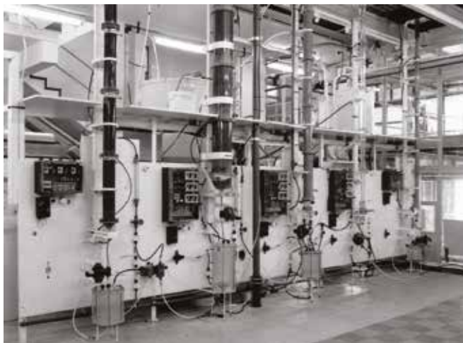
The ion-exchange columns which dominated the interior of the Chemical Engineering building for some years in the early 1970s. The multi-year effluent reclamation and desalination research project, funded by the WRC from 1972 – 1978, relied heavily on this experimental set-up.
