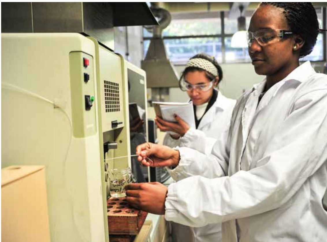
Jessica Heynes and Busisiwe May, both technical staff, working with the SpectrAA atomic absorption spectrometer in the Analytical Lab.
