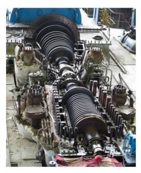
Steam turbines are some of the most commonly used machines for energy conversion and electricity generation. This focussed course will provide participants with an overview of their operation and how they can be modelled. The course will cover the steam turbine components as well as the associated feedwater heaters and condenser.
