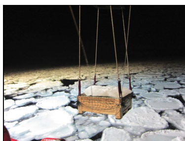
Fig 1: Basket lifting a pancake ice from the sea water
