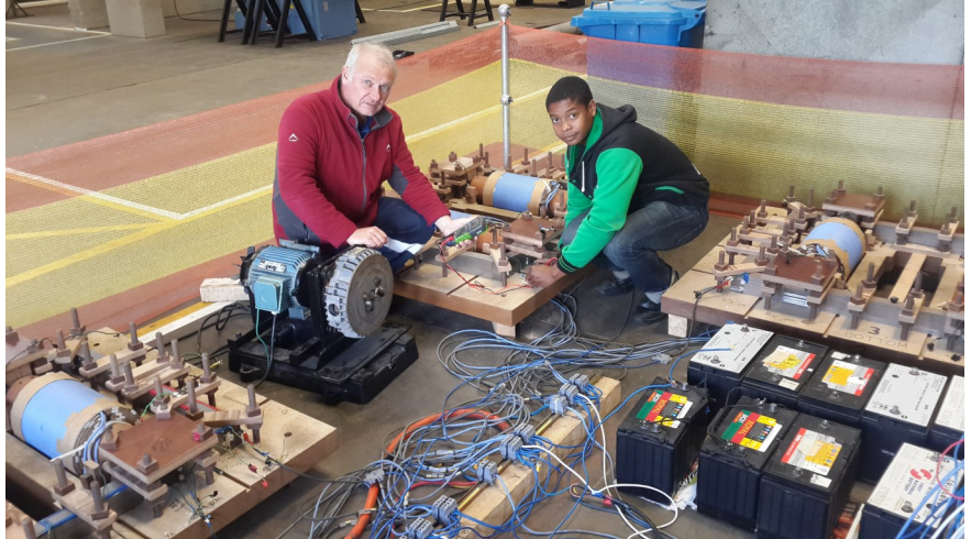
UCT doctoral students Les Borrill (left) and Hilary Chisepo (right) test model transformers to confirm the results of their simulations.
